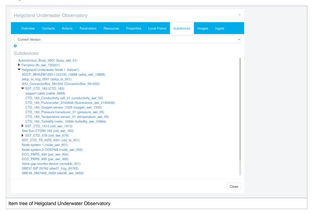
The tree-like structure can be seen under 'Subdevices'. By clicking on an entry in the tree a new window pops up showing the respective item.
