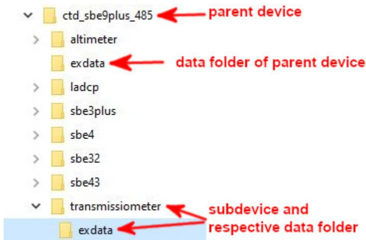
For every device operation you logged in DShip (see DShip stepwise manual under [DShip ActionLog manual](#)) on board during the expedition a folder with the device operation ID was attached to the 'exdata' folder of your device / subdevice. Raw data obtained during the specific device operation must be uploaded (automatically or manually by Data PI) to the respective subdirectory.
