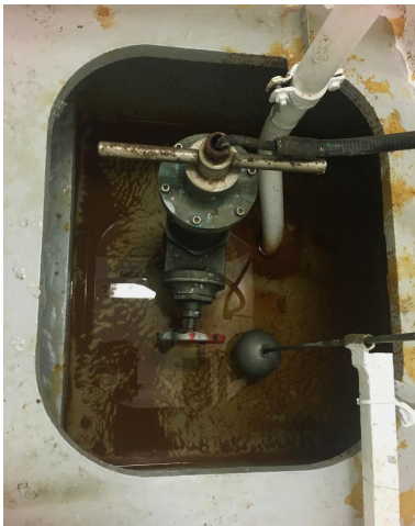
Installation of EM Log transducer in box keel
