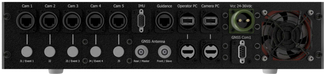
Figure 2: Computing unit rear panel
