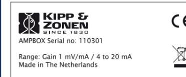
The standard AMPBOX gain setting is 1 mV/mA, so that 0 - 16 mV input gives 4 - 20 mA output
