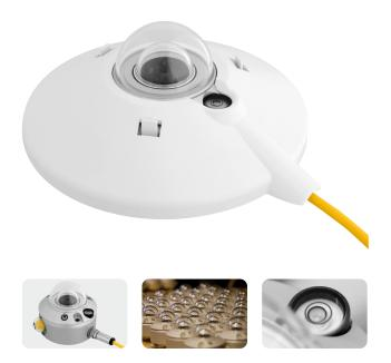
CMP 21 is similar to CMP 11 but has individually optimised temperature compensation. A standard thermistor sensor is fitted to monitor the housing temperature. Each instrument is supplied with its own temperature and directional (cosine) response data. It is the choice for scientific use and in top level solar radiation monitoring networks such as the Baseline Surface Radiation Network (BSRN) of the World Meteorological Organisation.
