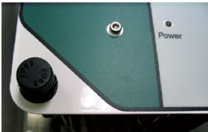
Figure 5-7. Unscrew the fuse cover to replace the fuse.
