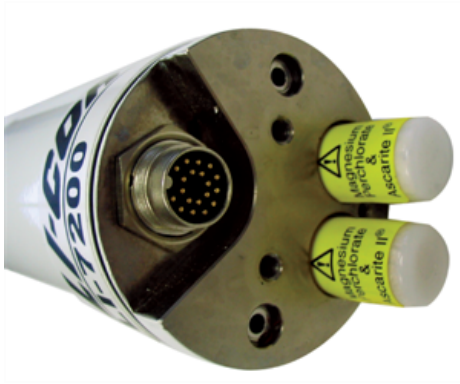
Figure 5-3. Insert the recharged bottles cap first. Make sure the caps have holes in the top.
