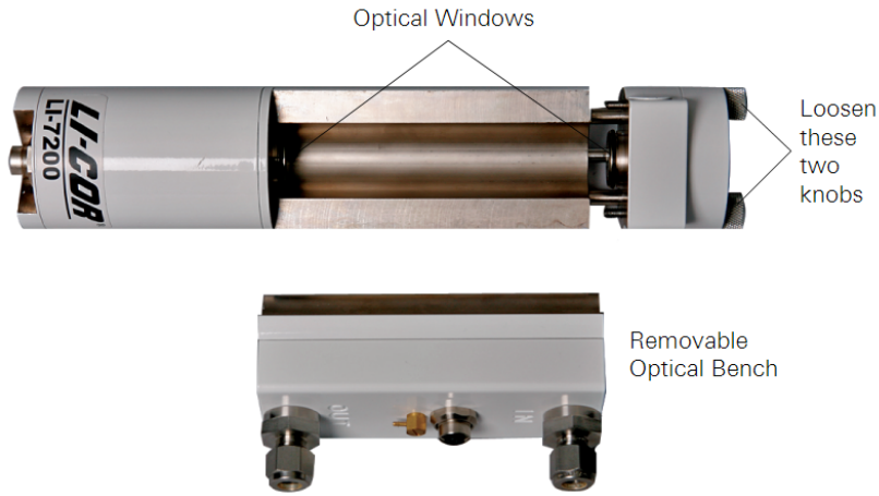
Figure 5-1. Slide the top end of the sensor head away from the bottom to remove the optical path.
