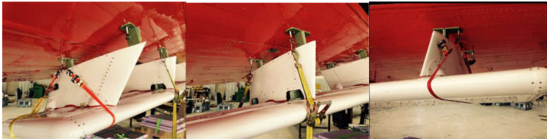
Figure 2-6: Wing Straps for Inboard, Mid and Outboard Pylons
