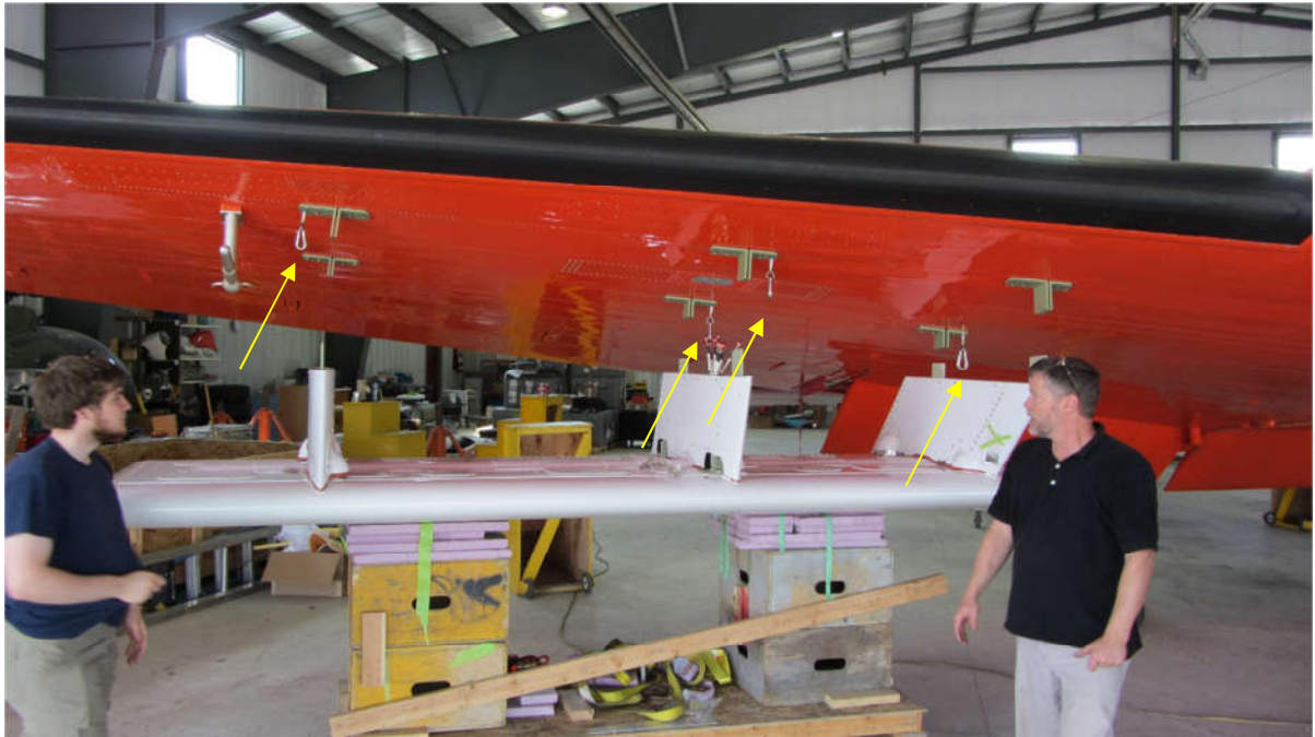
Figure 2-5: Shoulder Bolt Locations (note starboard wing shown)
