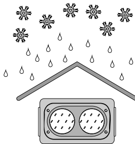
LD90-3 under a roof against rain, dripping water and snow fall
