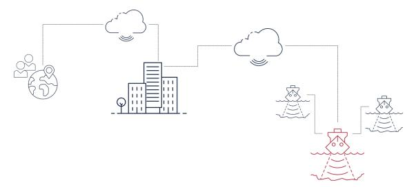
When SIS 5 Remote Operation is set up with a mothership, data from all survey launches are transmitted to the mothership. From there data from all EM-systems are sent to Blue Insight over an network connection. From Blue Insight the progress can be monitored from anywhere on the network.
