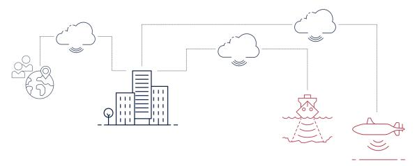
In autonomous mode there is no permanent network connection between SIS 5 on the boat and SIS 5 on shore. However, SIS 5 can be set up on the survey vessel to transmit some data at regular intervals to Blue Insight directly over an network connection. From Blue Insight the progress can be monitored from anywhere on the network. This provides the operator with a very good situation report to verify that the autonomous operation is going as planned.
