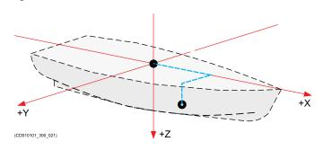
The accuracy of the three numerical values for X, Y and Z defines the accuracy of the sensor data. If you require a high accuracy, for example for underwater positioning, underwater mapping or scientific measurements, you must have each sensor positioned using professional land surveying. For such use, a good alignment survey is critical for high quality results. Surveys are normally done by qualified and trained surveyors using proven survey equipment and methods.
