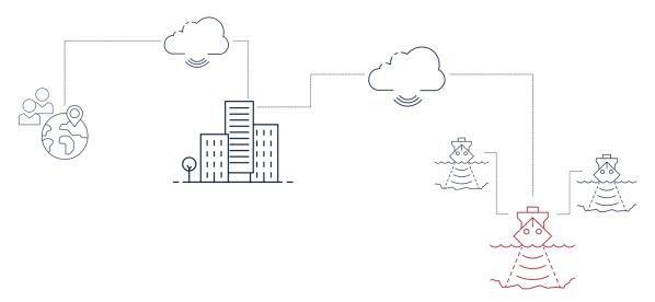
When SIS 5 Remote Operation is set up with a mothership, data from all survey launches are transmitted to the mothership. From there data from all EM-systems are sent to Mapping Cloud over an network connection. From Mapping Cloud the progress can be monitored from anywhere on the network.
