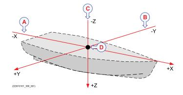
A positive value for X means that a sensor or a reference point is located <u>ahead</u> of the reference point (origin).
