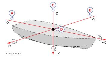
(y) position relative to the reference point. The coordinate system assumes that the x-axis follows the vessel's keel, and that the x-y plane is horizontal while the vessel is in normal trim.
