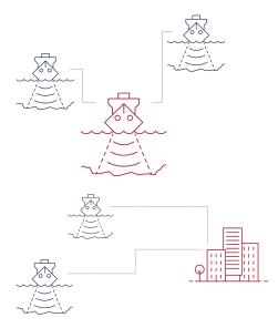
In both previous figures SIS 5 Server is installed on the survey vessels, and SIS Client is installed either on the mothership or on a PC on shore. In both cases the SIS 5 Client displays data from all survey vessels in the same display, and can control each EM-system independently. In this configuration a permanent network connection is assumed between SIS 5 Server on the launches and SIS 5 Client on the mothership or in shore.
