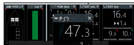
Figure 41 – Adding a measurement box to the panel. A white bar indicates where the box will be placed
