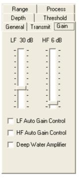
This is to manually set or adjust the gains on the LF and HF channels (range: 0 – 90 dB, steps: 1(9)dB). <u>Gains employed during data acquisition are final</u>. They are set by the hardware and cannot be changed during playback. For some SES-2000 systems there are other gain ranges or steps!
