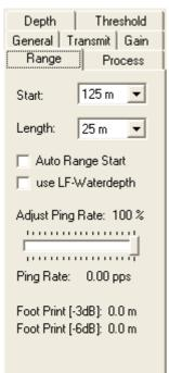
This defines the starting point and length of data to be recorded and <u>strongly affects the recorded data</u>: Any data outside of the specified window <u>will not be recorded</u>. The *Start* point and *Length* will vary depending on specific requirements of a survey.
