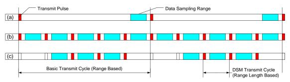
Principle of "Deep Sea Pulse Mode" and "Burst Pulse Mode":
