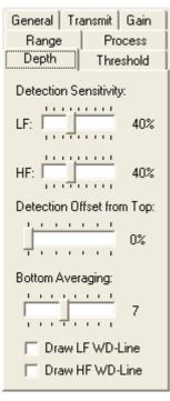
This affects the on-line depth calculation. Usually the default settings can be used: LF/HF Detection Sensitivity: 40% / 40% LF/HF Bottom Averaging: 5 - 7
