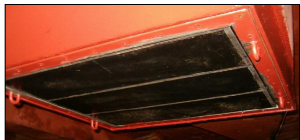
SES-2000 deep transducer mounted permanently in a streamlined dome below a ship's keel
