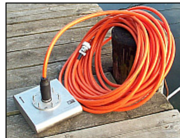
SES-2000 transducer with streamlined housing and supports to protect the active area (that is the blue area in the photograph).
