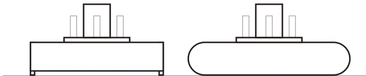
SES-2000 transducer with streamlined housing and supports to protect the active area (that is the blue area in the photograph).
