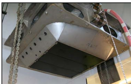
SES-2000 deep transducer prepared for moon-pool installation
