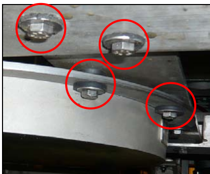
SES-2000 ROV transducer mounted using rubber to avoid any metal-metal connection.
