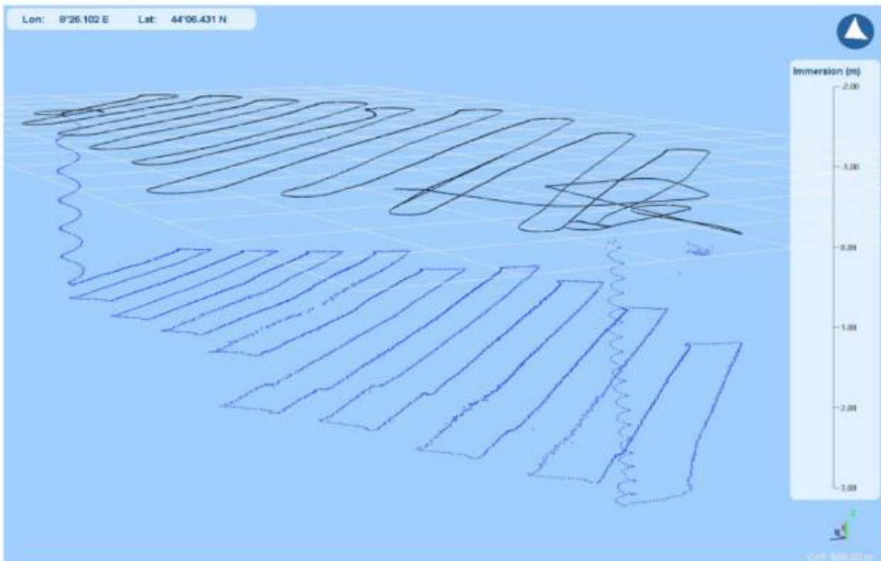
3D view of vessel trajectory (black) and ROV positions (blue)
