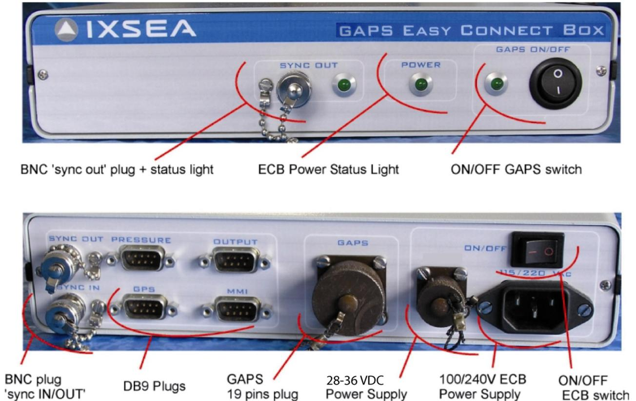
Figure 25 - ECB Box, Front Face and Back Face
