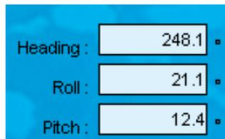
*This test is successful if you can monitor the heading, roll and pitch in the GAPS MMI software.*
