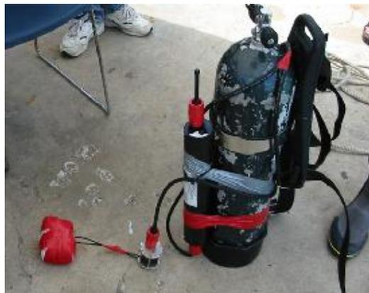
Figure 21 - Transponder fixed on a scuba cylinder
