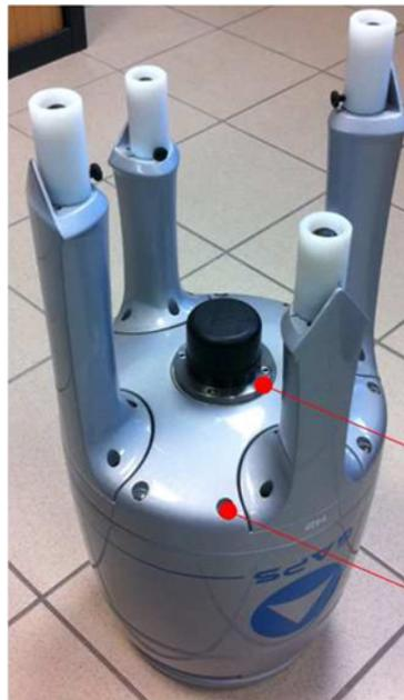
If the voltage between the GAPS antenna and the hull of the ship is below 1.0 V, the system is electrically well installed.
