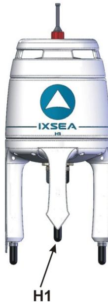
Figure 16 - GAPS H1 hydrophone location
