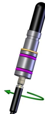
9. Screw the new hydrophone to the connector.
