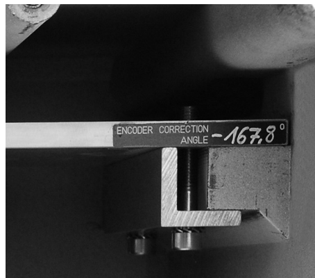
Figure 6-2: Shaft encoder correction angle value sticker
