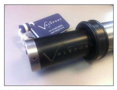
On first installation, it will require 2 mins initialise, during this period the magnetic switchkey should be removed.
