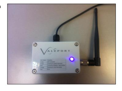
The receiver will install as a USB serial port adaptor and should install automatically on most windows PC's. If the receiver will not automatically install, drivers can be downloaded from:
