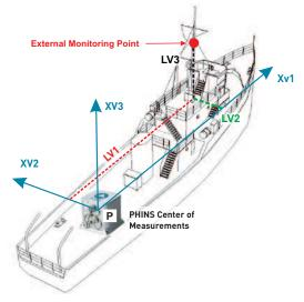
Figure 2 - Definition of lever arm
