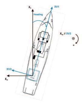
Once the axes XV2 and XV1 lie in the local horizontal plane, the true heading is the angle between the vertical plane oriented in the North direction and the vertical plane passing through the vessel. Heading is counted positive from North, varying from 0 to 360∞. The orientation of this angle is given above in case of null pitch and roll.
