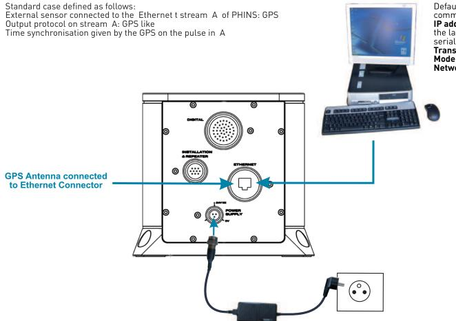
Default Settings for an Ethernet communication PC <-> PHINS: IP address:192.168.36.1xx, xx being the last two numbers of the PHINS
