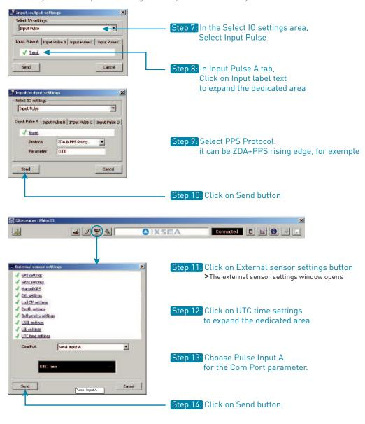
Note: Send command stores the configuration into the PHINS non volatile memory
