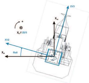
The roll is defined as the angle of rotation perform around the vessel XV1 so that the vessel axis XV2 lies in the local horizontal plane. This angle is default defined positive in the direction of axis XV1, i.e., when the boat port side is up. It varies between -180 and + 180. The figure above is an illustration of the roll angle with null pitch.
