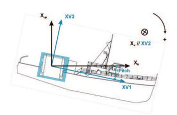
Once the axis XV2 lies in the local horizontal plane, the pitch is the angle between the axis XV1 of the vessel and its projection in the local plane. This angle is default defined positive in the direction of axis Xv2, i.e., When the boat bow is down. It varies from -90 to  $+90\infty$ . The figure above is an illustration of the pitch angle in case of null roll
