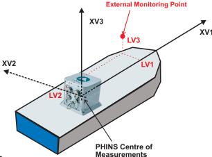
Figure 2 - Definition of lever arm
