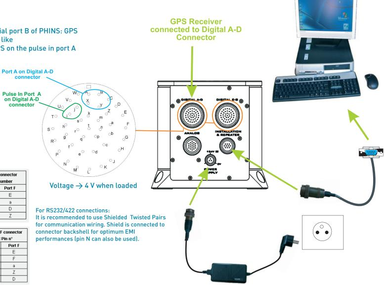
As soon as PHINS is powered up it starts its alignment phase starting with the manually input position stored into PHINS PROM. It is required that a valid initial position is input manually (see section Step 3) or is given by the GPS. The alignment sequence is detailed in Step 4.
