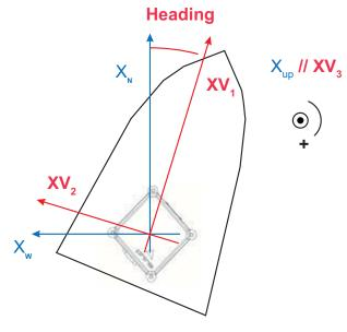
The roll is defined as the angle of rotation perform around the vessel XV1 so that the vessel axis XV2 lies in the local horizontal plane. This angle is default defined positive in the direction of axis XV1, i.e., when the boat port side is up. It varies between -180 and  $+180\infty$ . The figure above is an illustration of the roll angle with null pitch.
