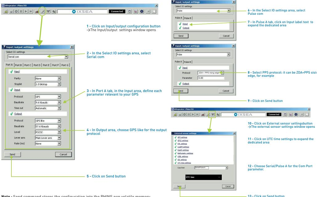
Note: Send command stores the configuration into the PHINS non volatile memory
