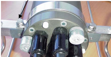
Hex head screw and washer (2 on each clamp, clamps top and bottom of housing)
