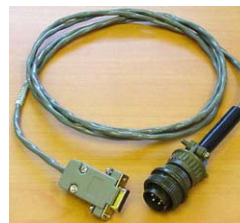
CDO Remote Out Interface test cable
