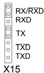
FIGURE 4-2 RS 232C/TTL level and phase selections
