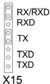
FIGURE 8-2 Basic RS 232C settings
