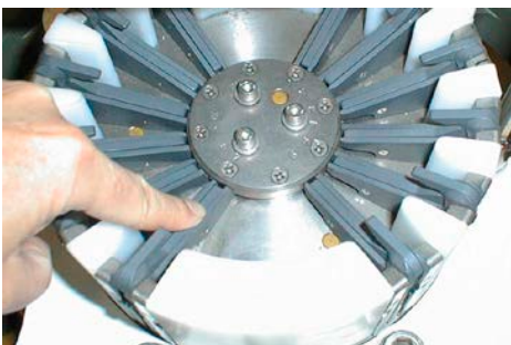
Push trigger to cock release mechanism
