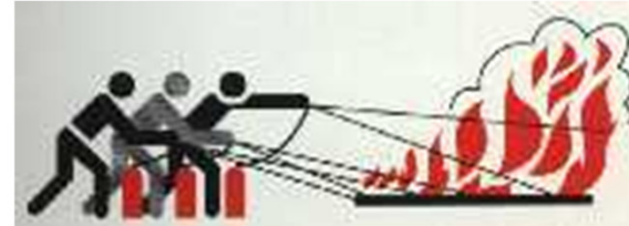
Use several fire extinguishers at the same time
