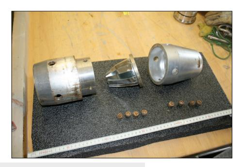
**Details of the Core Bit & Core Catcher**
