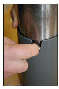
Insertion of steel spheres
