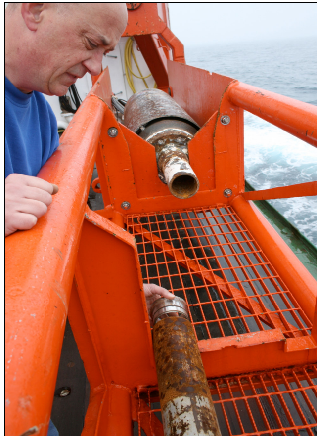
The four-metre tube being installed at the lower weight unit
