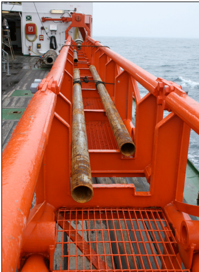
Core frame with steel-core tubes, 105 mm in diameter (lengths: 4 m, 5 m, 1 m)
