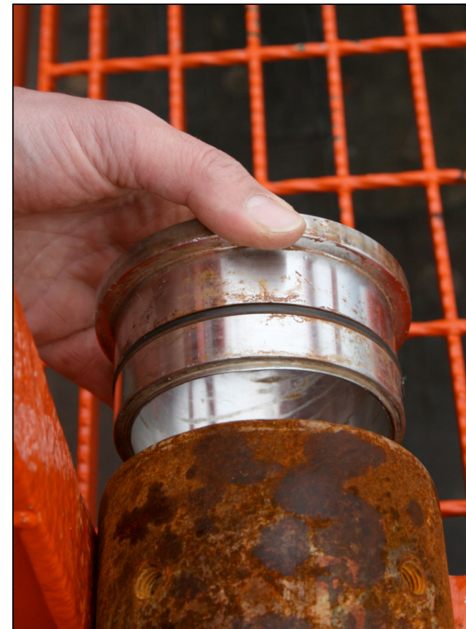
Connection piece to weight unit at top of uppermost core tube
