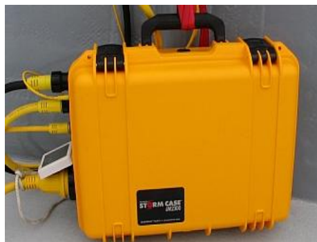
Figure 5 UCTD power supply with all cables attached.
