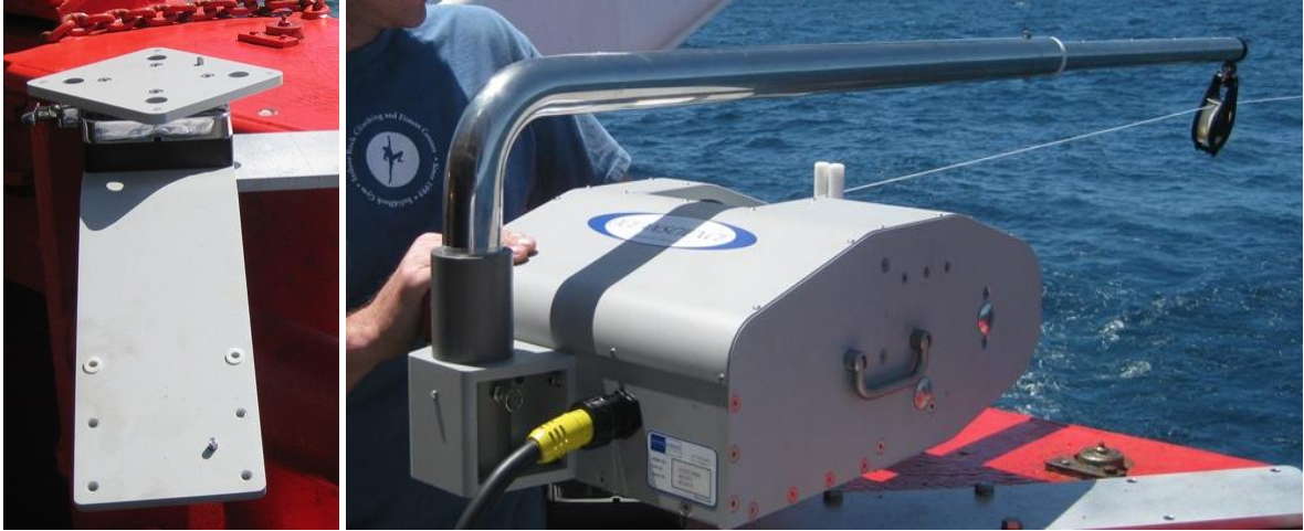
Figure 4 Rewinder and winch mounts (left) on the gunwale at the stern of a vessel. Davit arm mounted to the UCTD winch (right).
