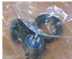
4-pin MS connector assembly (for SEACAT data I/O connector on Interface Box)
