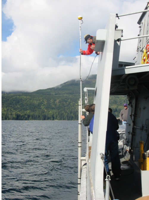
Figure 25 - DGPS antenna installation
