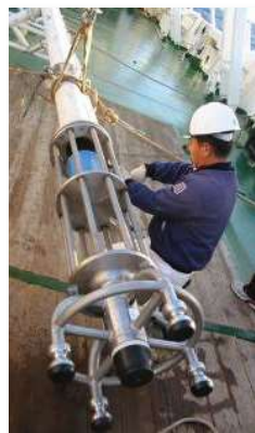
Deployable array and OCTANS on side pole.
