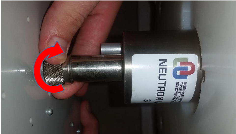
Figure 10: MiniNM head removal
