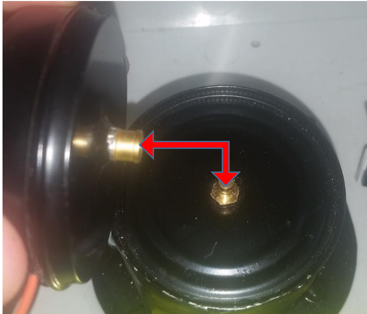
Figure 15: SMB connector alignment
