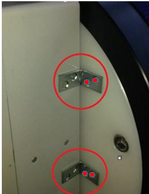
Figure 9: L-Bracket screws to be removed.
